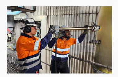
HRL engineers undertaking online particle sizing measurement using a specialist probe.
