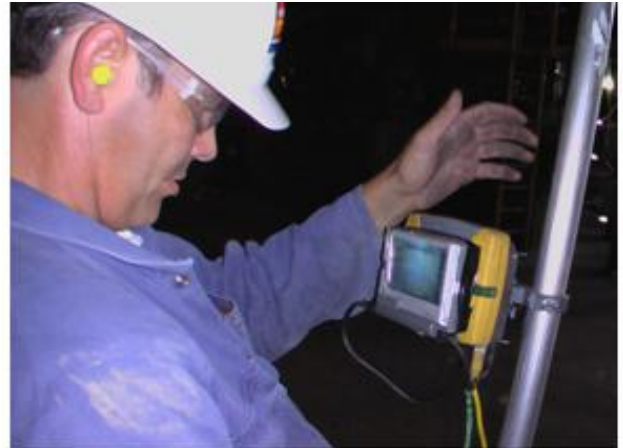
An imaging device is used to capture readings from difficult-to-access hangers.
